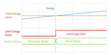
Parameter No. 43 (0x2B): Energy Level (4 byte) – Sets the energy level that once exceeded an Energy Limit event occurs.
