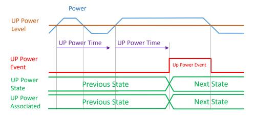
Parameter No. 35 (0x23): UP Power Level (2 byte) – Sets the level of instantaneous power in Watts beyond which time of permanence above this level is calculated.
