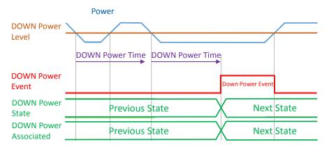
Parameter No. 39 (0x27): DOWN Power Level (2 byte) – Sets the level of instantaneous power beyond which the time of permanence below this level is calculated.
