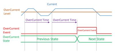
Parameter No. 30 (0x1E): Overcurrent level (2 byte) – Sets the current level above which the time spent above that level is measured.
